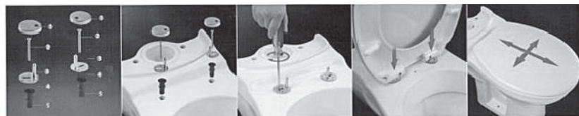
Hinge set. 1) Insert the hinges into the toilet. 2) Tighten the screws of the hinges. Do not over tighten. 3) Insert the seat cover onto the toilet. 4) Align the toilet seat and cover with ceramic.
